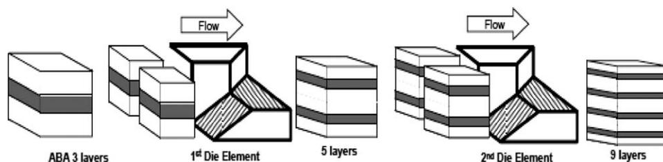
Figure 1 Layer-multiplying coextrusion for forced-assembly of polymer nanolayers.
