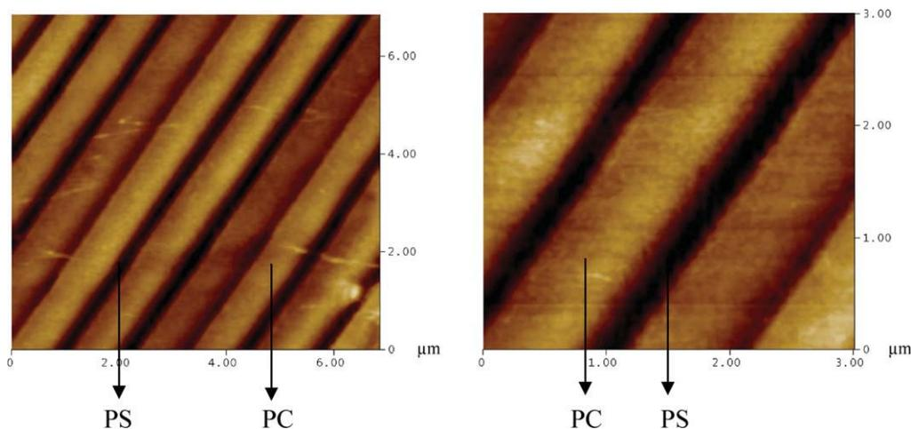
**Figure 2** AFM images of PC/PS 70/30 125  $\mu\text{m}$  thick multilayer film (left image: low magnification image; right image: higher magnification image). [Color figure can be viewed in the online issue, which is available at [wileyonlinelibrary.com](http://wileyonlinelibrary.com).]
