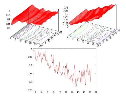
Figure 3: Bottom changes minimizing  $J_2$  after 20 hours starting from a linear bottom. Water elevation (upper/left), bathymetry (upper/right) and evolution of the normalized cost function in time (lower).
