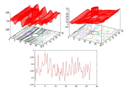
Figure 4: Bottom changes minimizing  $J_2$  starting from a linear bottom plus an immersed cylindrical structure. Water elevation (upper/left), bathymetry (upper/right) and evolution of the normalized cost function in time (lower).
