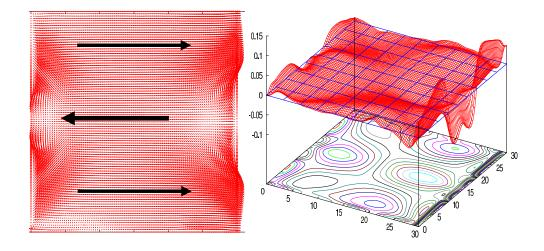
Figure 5: Finding a bottom surface (right) generating a target mean current (left). On the flat bottom the mean current is zero. The flow elevation is periodic and prescribed on the left boundary. The final shape is far from being intuitive.
