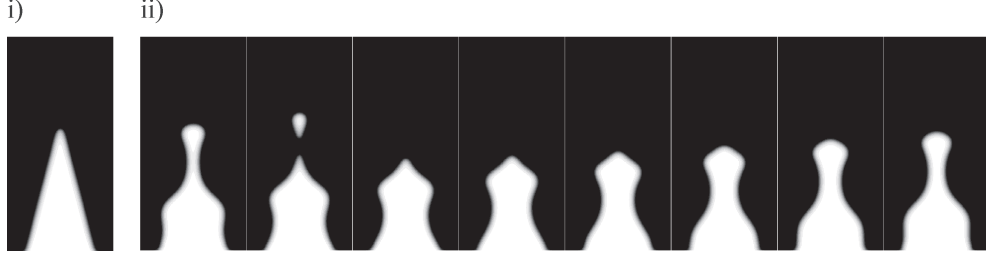
FIGURE 2. Instantaneous field of mass fraction burnt thresholded at 50% for i) St = 1 and ii)
