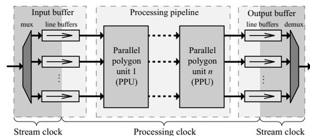
Fig. 12 Overall architecture of parallel ASF application.
