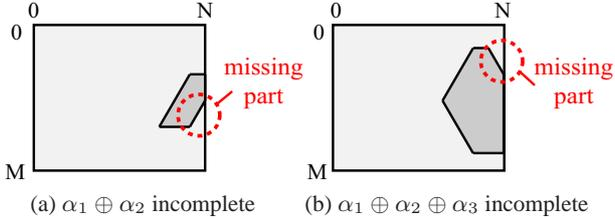
**Fig. 3** Polygon SE composition without padding. The desired SEs presented in Fig. 2 are incomplete, a small triangle is missing.
