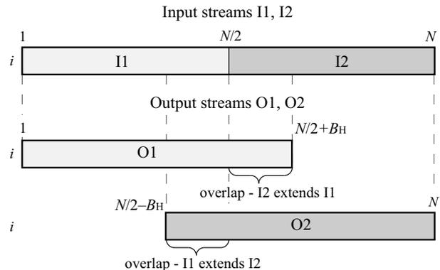
Fig. 11 Addition of overlap on one image line
