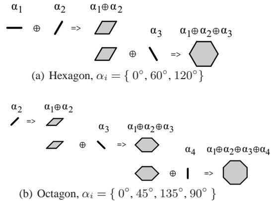
**Fig. 2** Polygon SE composition of line SEs. (a) hexagon is composed of 3 segments, (b) octagon is composed of 4 segments.  $\oplus$  operator stands for the Minkowski addition;  $\alpha_i$  stands for  $L_{\alpha_i}$ .
