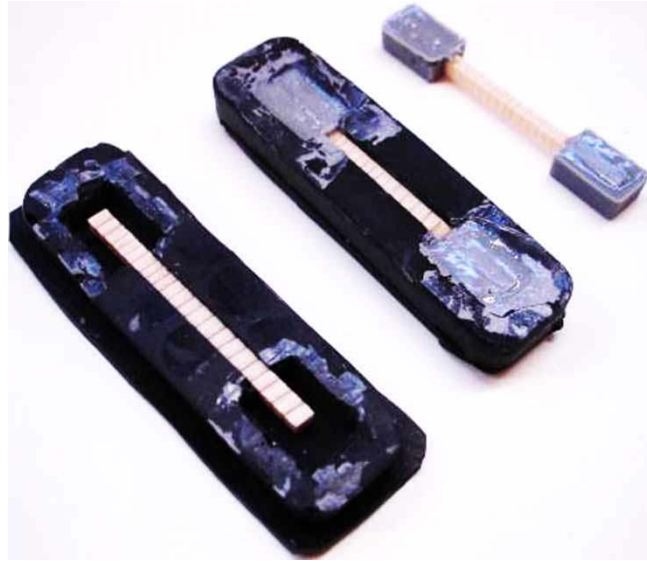
Figure 1. Sample preparation: embedding of the two ends of the samples in epoxy resin with a silicone mould. The dimension of the samples was 50 \times 3 \times 3 mm (radial \times tangential \times longitudinal).
