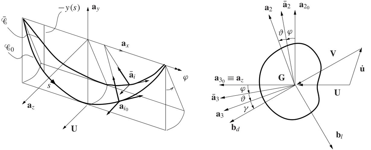
**Figure 2.** Aerodynamic forces. Left: cable configuration. Right: transversal section, mean wind velocity  $\mathbf{U}$ , relative wind velocity  $\mathbf{V}$ , angle of attack  $\gamma$ , drag force  $\mathbf{b}_d$  and lift force  $\mathbf{b}_l$ .
