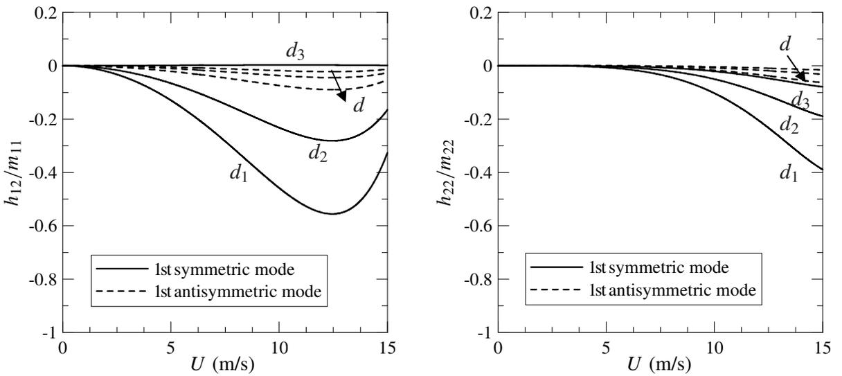
**Figure 8.** Coefficients of the circulatory matrix  $\mathbf{H}$ : left, coupling terms; right, terms modifying the structural stiffness ( $d_1 = 3$  m;  $d_2 = 6.18$  m;  $d_3 = 15$  m;  $\ell = 267$  m; CS1).
