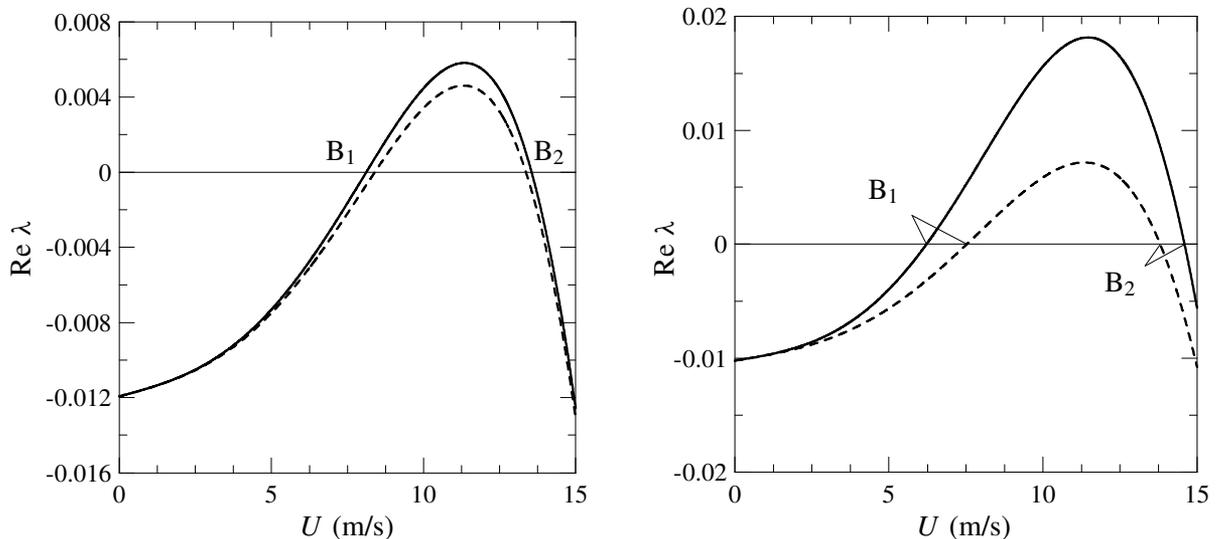
**Figure 10.** Real part of the critical eigenvalue of the CS2: left,  $d = 6.18$  m; right,  $d = 3$  m (sectional symmetry axis rotated through  $-47^\circ$  in no-wind conditions). Continuous lines, complete model; dashed lines, matrix  $\mathbf{H}$  neglected.
