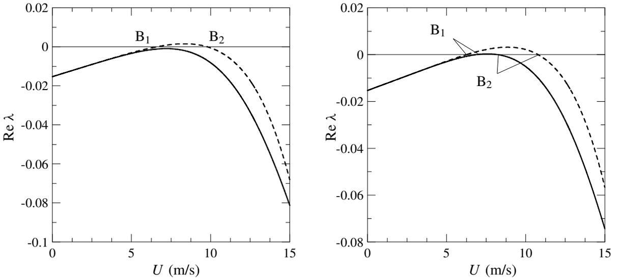
**Figure 9.** Real part of the critical eigenvalue of the CS1: left,  $d = 3$  m; right,  $d = 3$  m and sectional symmetry axis rotated through  $-1^\circ$  in no-wind conditions (damping coefficients equal to 0.65%). Continuous lines, complete model; dashed lines, matrix  $\mathbf{H}$  neglected.
