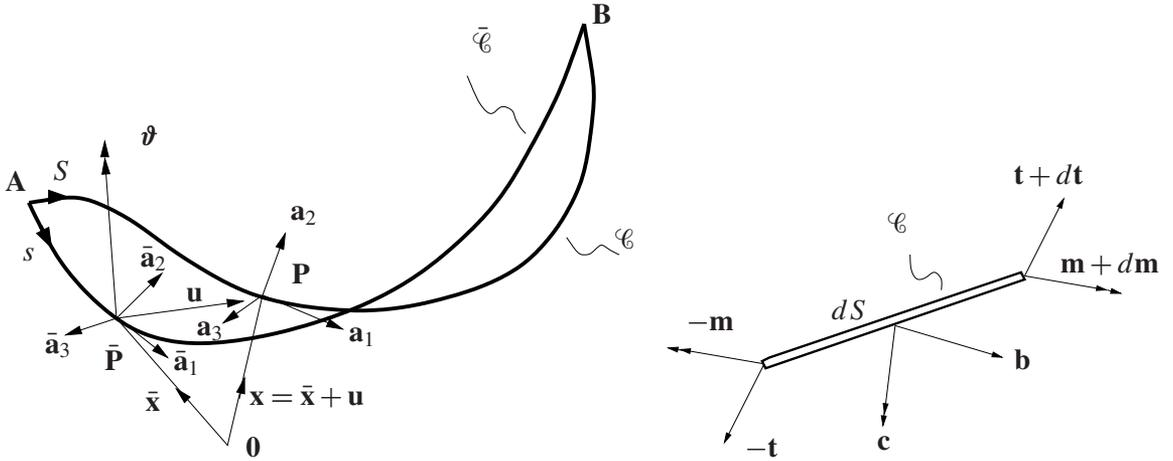
**Figure 1.** Left: configurations of the cable. Right: forces and couples on an infinitesimal element.
