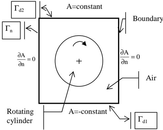
**Fig. 1.** Rotating cylinder in a constant magnetic field
