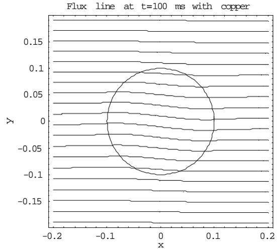
**Fig. 5.** Flux lines obtained with finite element simulation.
