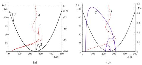
**Figure 3.** Landslide motion over an uneven bottom of the model reservoir. (a): *I*, *2* form of landslide at the initial time moment (*I*) and at the stop moment for  $\theta_* = 5^\circ$  (*2*); *3*, *4* graphs of the function  $x = x_c(t)$  for  $\theta_* = 5^\circ$  (*3*) and  $\theta_* = 1^\circ$  (*4*); (b): graphs of the function  $x = x_c(t)$  (*I*) and the dependence of the Froude number *Fr* on the coordinate  $x_c(t)$  (*2*) for  $\theta_* = 1^\circ$ .
