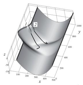
Figure 1. Landslide motion trajectory for two different start positions:  $l - x_c^0 = 91.5 \text{ m}, y_c^0 = 620 \text{ m};$  $2 - x_c^0 = 115.2 \text{ m}, y_c^0 = 660 \text{ m}.$
