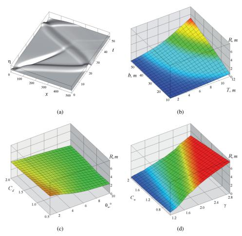
**Figure 4.** Graph of the surface  $z = \eta(x,t)$  (a) and graphs of dependences of the maximal splashing *R* on the length *b* and height *T* of the underwater landslide (b), on the resistance coefficient  $C_d$  and the angle of friction  $\theta_*$  (c), on the coefficient of associated mass  $C_w$  and relative density of landslide mass  $\gamma$  (d).
