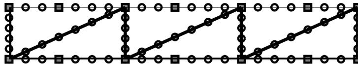
Figure 1. Finite element mesh of the truss. Symbol  $\circ$ : nodes of the mesh, symbol  $\square$  measured nodes, thick solid line: elements with fixed properties, thin solid line: elements whose properties have to be updated.
