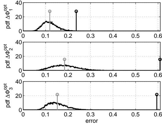
Figure 5. Updated uncertain computational model corresponding to  $(s^{opt}, \delta^{fix}) = (26.2, 0.3)$ . Graph of the probability density functions  $\Delta\tilde{\Phi}_\alpha^{opt}$  (black line), of its first order moment  $\mathcal{E}\{\Delta\tilde{\Phi}_\alpha^{opt}\}$  (vertical gray line), of  $\Delta\tilde{\phi}_\alpha^{ini}$  (vertical black line) for  $\alpha = 1$  (upper graph),  $\alpha = 2$  (middle graph),  $\alpha = 3$  (lower graph).
