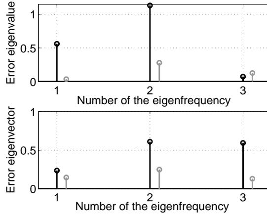
**Figure 2.** Quantification of the errors between the non updated and the updated mean computational model with the experimental data. Upper graph : graph of  $\alpha \mapsto \Delta \underline{\lambda}_\alpha^{ini}$  (black line),  $\alpha \mapsto \Delta \underline{\lambda}_\alpha^{opt, det}$  (gray line). Lower graph : graph of  $\alpha \mapsto \Delta \underline{\phi}_\alpha^{\tilde{ini}}$  (black line),  $\alpha \mapsto \Delta \underline{\phi}_\alpha^{\tilde{opt, det}}$  (gray line).
