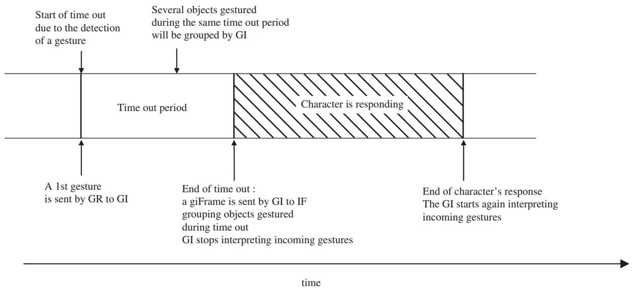
Fig. 4. Temporal management in the GI module.
