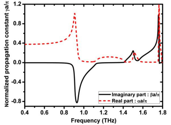
FIG. 5. Dispersion diagram of a symmetrical fishnet array designed for an operating frequency of 1 THz:  $d_x = d_y = 170 \mu\text{m}$ ,  $a_y = 58 \mu\text{m}$ ,  $EAR = 2$ , and  $d_z = 13 \mu\text{m}$ .
