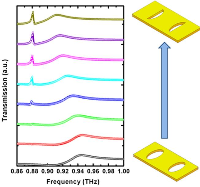
FIG. 7. Transmission curves reported on a shifted scale versus frequency when the elliptical apertures are progressively closed.
