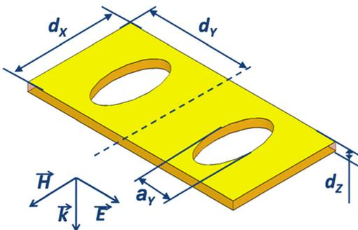
FIG. 1. Unit cell of the metamaterial sensing structure:  $d_x = d_y = 170 \mu\text{m}$ ,  $EAR = 2$ , metal thickness =  $0.4 \mu\text{m}$ , BCB interlayer =  $13 \mu\text{m}$ . Inset: Schematic of the polarization configuration.
