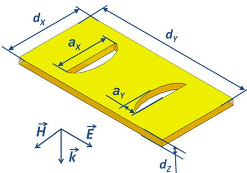
FIG. 8. Unit cell of the HE metamaterial structure:  $d_x = 170 \mu\text{m}$ ,  $d_y = 340 \mu\text{m}$ ,  $a_y = 29 \mu\text{m}$ ,  $a_x/a_y = 4$ , metal thickness =  $0.4 \mu\text{m}$ , BCB interlayer =  $13 \mu\text{m}$ . Inset: Schematic of the polarization configuration.
