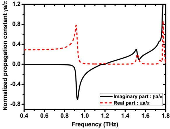
FIG. 3. Dispersion diagram of a symmetrical fishnet array designed for an operating frequency of 1 THz:  $d_x = d_y = 170 \mu\text{m}$ ,  $a_y = 76 \mu\text{m}$ ,  $EAR = 2$ , and  $d_z = 13 \mu\text{m}$ .
