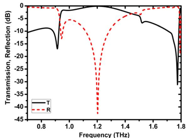
FIG. 2. Reflection and transmission spectra of a symmetrical fishnet array designed for an operating frequency of 1 THz:  $d_x = d_y = 170 \mu\text{m}$ ,  $a_y = 76 \mu\text{m}$ ,  $EAR = 2$ , and  $d_z = 13 \mu\text{m}$ .
