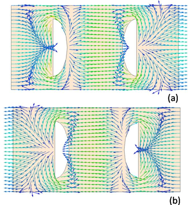
FIG. 17. Surface current plots on the top face (a) and bottom face (b) of the BCB interlayer at 0.885 THz.
