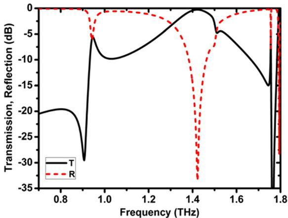
FIG. 4. Reflection and transmission spectra of a symmetrical fishnet array designed for an operating frequency of 1 THz:  $d_x = d_y = 170 \mu\text{m}$ ,  $a_y = 58 \mu\text{m}$ ,  $EAR = 2$ , and  $d_z = 13 \mu\text{m}$ .
