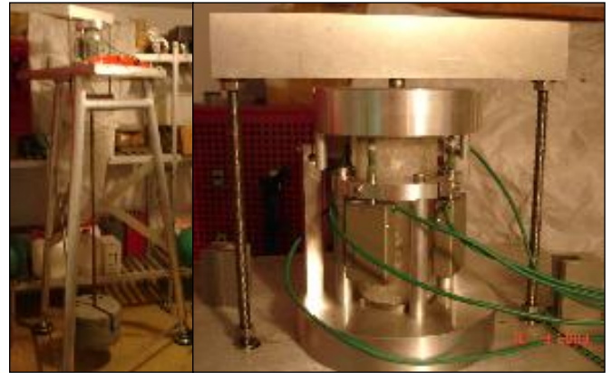
Figure 3. Testing device and salt sample below the upper plate.
