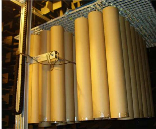
**Figure 1.** (Color online) Experimental set up. Picture of the frame in which the SCW has been hung and the complete structure with  $7 \times 7$  rows in which the central one is removed in order to produce the waveguide.
