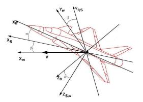
Fig. 1. Frames: Body fixed axes  $OX_BY_BZ_B$ , Stability axes  $OX_SY_SZ_S$ , Aerodynamic axes  $OX_WY_WZ_W$
