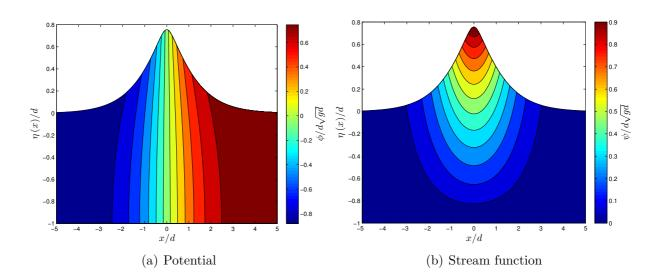
**Figure 7.** Equi-potentials (left) and iso-stream-function (right) under a large wave. Lines correspond to the iso-values computed in the 'fixed' Frame of reference where the the fluid is at rest in the far field  $x \to \pm \infty$ .
