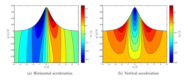
Figure 10. Iso-horizontal (left) and iso-vertical (right) accelerations under a large wave.
