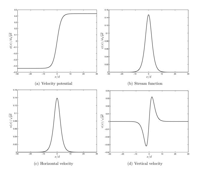
Figure 3. The velocity potential, stream function, horizontal and vertical velocities evaluated at the free surface for the Froude number  $F_{\text{TAN}} =$ 1.066365888477383. (Note the different scales between the plots.)
