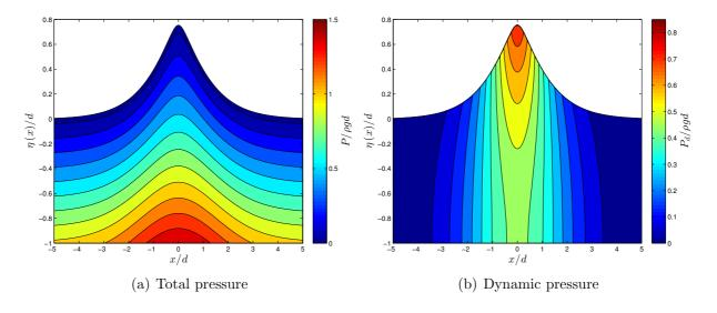
Figure 8. Isobars (left) and iso-dynamic-pressures p + gy (right) under a large wave.
