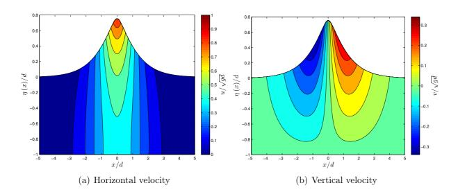
Figure 9. Iso-horizontal (left) and iso-vertical (right) velocities under a large wave. Lines correspond to the iso-values computed in the 'fixed' Frame of reference where the the fluid is at rest in the far field  $x \to \pm \infty$ .
