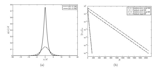
Figure 4. Two solitary waves computed in multiprecision arithmetics along with the convergence curves showing the decay of the error in  $L_{\infty}$  norm.
