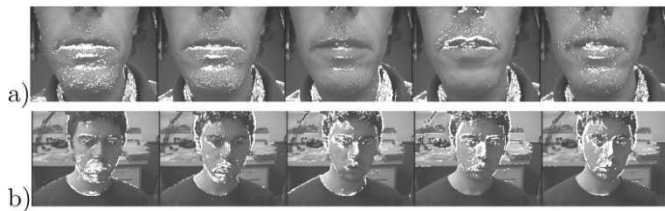
Fig. 6. Temporal changes detected by entropic thresholding: (a) micro-camera centered on the lower part of the face and (b) webcam sequence in office room.
