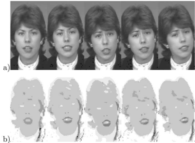
Fig. 7. Face Segmentation: (a) sample frames of color video sequence Claire and (b) label fields after relaxation, with gray levels coding the hue clusters.
