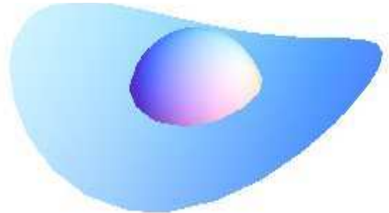
FIG. 1: Three-phase boundary of a spherical particle at a liquid interface with curvatures c_2 = -\frac{1}{2}c_1 . The contact line is not a circle but undulates in space.
