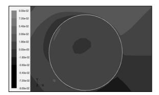
Figure 24. Tangential Velocity-z=0.25D-case II
