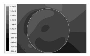
Figure 22. Tangential Velocity-z=0.125D-case II
