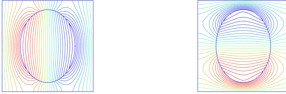
Figure 11.2: Potentials V_x (left) and V_y (right): The unit cell contains an elliptic inclusion of relative permittivity ( \epsilon = 4.0 + 3i ) with minor and major axis a = 0.3 and b = 0.4 in silica ( \epsilon = 1.25 ).
