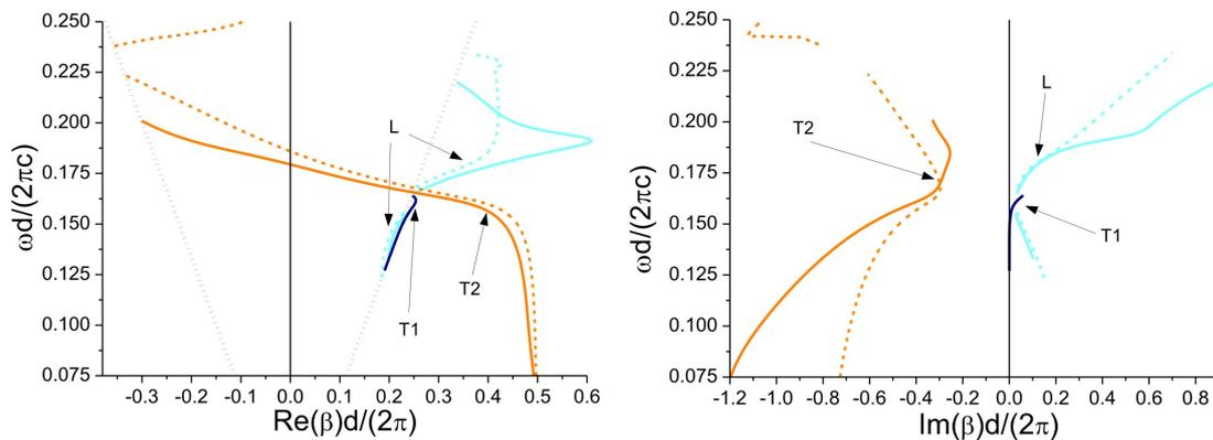
Figure 6.2: Real and imaginary parts of the dispersion relations in the dipole approximation (dashed curves), and fully converged multipole calculations with  $n_{\text{max}} = 10$  (full lines). The Longitudinal mode with positive imaginary part is in cyan(gray) the “T1” mode with positive imaginary part is in blue(black line). The “T2” transverse mode with negative imaginary part is in orange(gray). reproduced with permission : <http://dx.doi.org/10.1364/JOSAB.29.001012>
