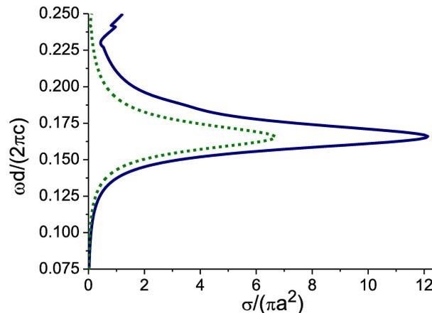
Figure 6.3: Normalized extinction is a solid blue (line) and scattering cross section given by a dashed green line of a silver monomer in terms of frequency ( $a = 25\text{nm}$ ). reproduced with permission : <http://dx.doi.org/10.1364/JOSAB.29.001012>
