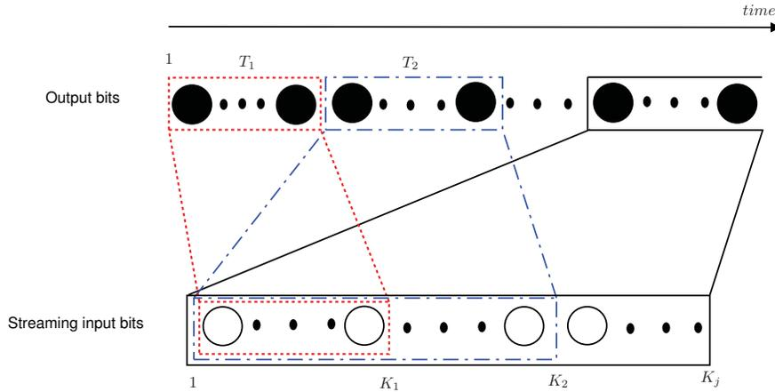
Figure 22: Anytime UEP-LT encoding scheme.
