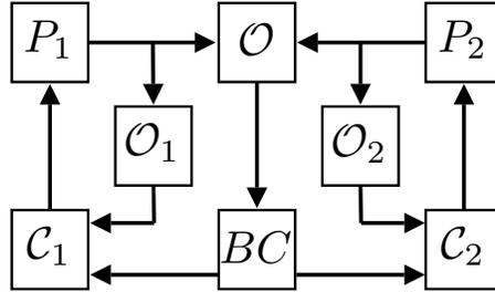
Figure 19: Two plant setup ( $P_1$  and  $P_2$ ) each with a controller ( $C_1$  and  $C_2$ ), a joint observer ( $O$ ), which observes both plant states, and individual observers ( $O_1$  and  $O_2$ ), which observe one plant state each. The joint observer communicates its observation to the two controllers using a wireless broadcast channel (BC).
