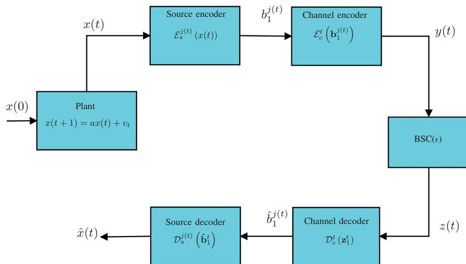
Figure 21: The functional diagram of a dynamic system using an anytime code.
