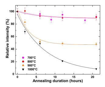
Fig. 4. Relative intensity of the (002) XRD AIN peak as a function of the annealing duration
