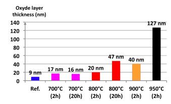
Fig. 7. Thickness (±2 nm) of the oxide overlayer determined by ellipsometry for different samples
