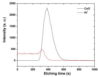
Fig. 5. SIMS depth profile signal of an AIN/Sapphire sample after a 2h long annealing process. A thin conductive Pt layer was sputtered at the surface to reduce charging effects.
