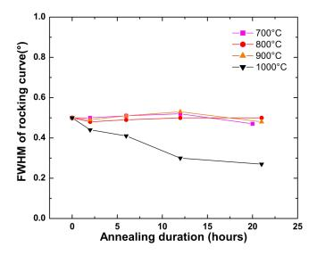
Fig. 1. FWHM of the rocking-curve of AIN (002) as a function of the annealing duration
