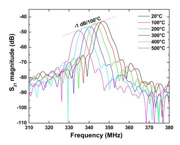
Fig.9. |S<sub>21</sub>| signal of IDT (Pt/Ta)/AIN/Sapphire SAW delay line from 20 to 500°C
