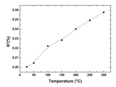
Fig. 10. Evolution of K<sup>2</sup> of AIN/Sapphire structure with temperature
