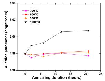
Fig. 2. c-lattice parameter of the AIN film as a function of the annealing duration
