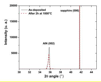
Fig. 3. θ-2θ XRD scan mode of as-prepared and 2h annealed AIN/Sapphire samples
