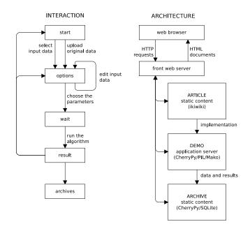
Fig. 1. Workflow and design of the web demo system.
