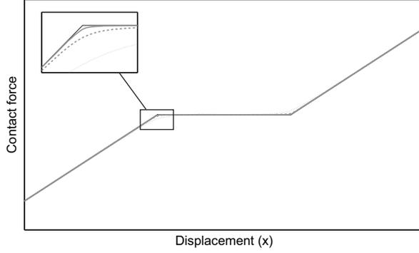
**Fig. 3.** Comparison of the piecewise-linear contact force obtained with Eq. (2) (in black) and the regularized contact force obtained with Eq. (9) (in grey) for different values of  $\eta$ . Parameter values:  $\alpha=30$ ,  $\eta=0.005$  (solid line),  $\eta=0.05$  (dashed line),  $\eta=0.5$  (dotted line).
