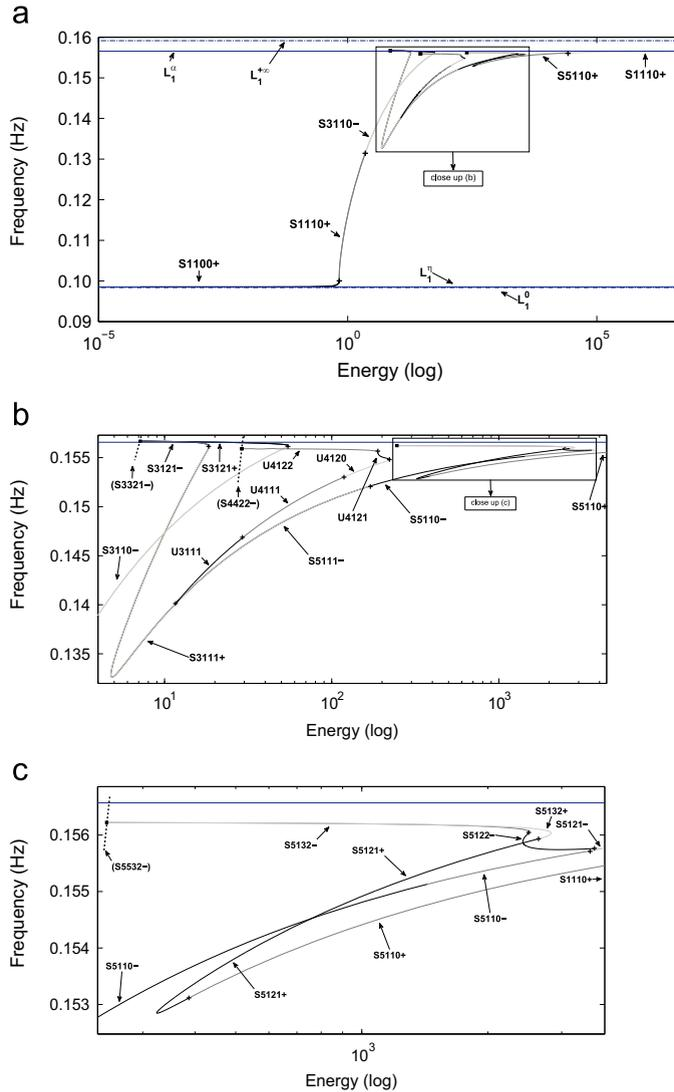
**Fig. 8.** FEP of the in-phase NNM: (a) overview, (b) and (c) close ups. The black square markers indicate internal resonances. The black plus markers indicate the change of branches. (Parameter values:  $\alpha=30$ ,  $\beta=1$ ,  $\delta=1$ ,  $\eta=0.005$ ,  $H=33$ ,  $H_f=151$ .)
