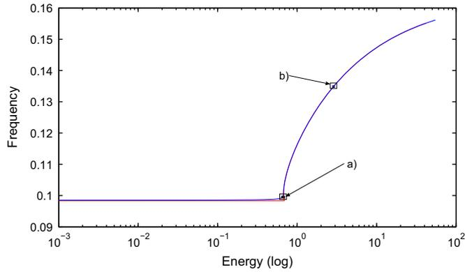
**Fig. 4.** FEP corresponding to the first NNM of the non-smooth system obtained from direct computation (in red) and from the HBM-ANM method (in blue). (Parameter values:  $\alpha=30$ ,  $\beta=1$ ,  $\delta=1$ ,  $\eta=0.005$ ,  $H=33$  and  $H_f = 151$ .) (For interpretation of the references to color in this figure caption, the reader is referred to the web version of this paper.)
