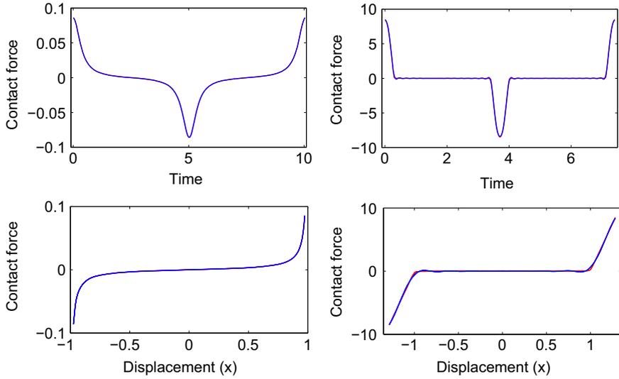
**Fig. 6.** Contact force for points (a) and (b) in Fig. 4 given by Eq. (9) (in red) and obtained from the HBM-ANM method (in blue). First row: time evolution over one period, second row:  $(x, f(x))$ -plot. (Parameter values:  $\alpha=30$ ,  $\beta=1$ ,  $\delta=1$ ,  $\eta=0.005$ ,  $H=33$  and  $H_f = 151$ .) (For interpretation of the references to color in this figure caption, the reader is referred to the web version of this paper.)
