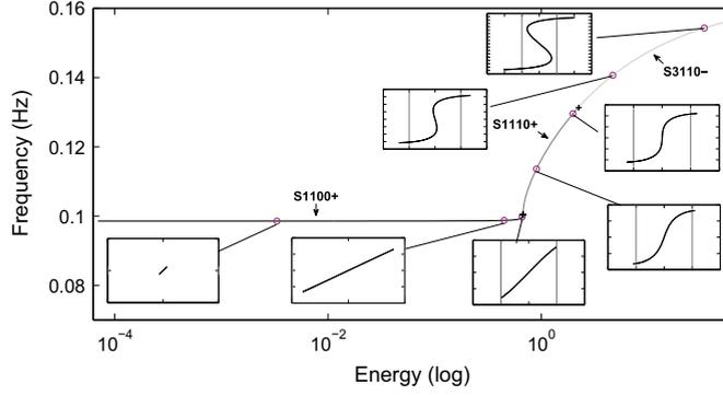
**Fig. 9.** Zoom on particular branches (S1100+, S1110+, S3110-) of the FEP of the in-phase NNM, some periodic orbits are represented by modal line (see the boxes). The black plus markers indicate the change of branches. (Parameter values:  $\alpha=30$ ,  $\beta=1$ ,  $\delta=1$ ,  $\eta=0.005$ ,  $H=33$ ,  $H_f=151$ .)
