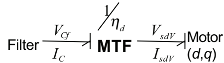
Fig. 17. Simple BG of the inverter for the induction motor modelled on the (d_v, q_v) reference frame.
