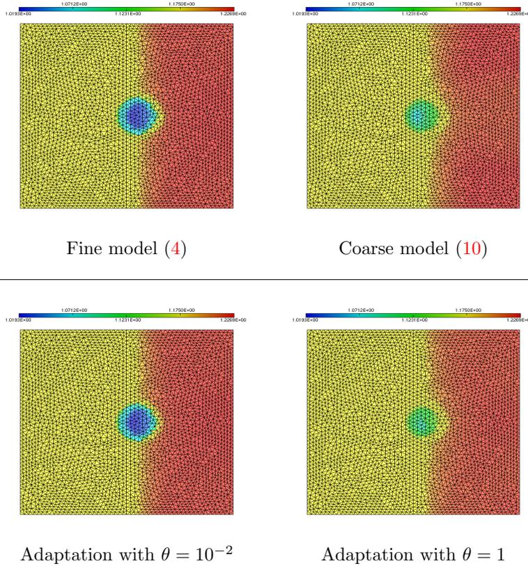
FIGURE 7. Shock bubble interactions. Solution during the second interaction: density  $\rho$
