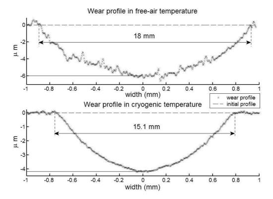
Figure 9: Rolling zone profile for disc 1 after the experiment for N = 72N in ambient air (top) and in Liquid nitrogen condition (bottom). One can see that wear depth is lower for cryogenic condition than for ambient air condition, which is easily justified by the lower value of the mean coefficient of friction during that test and the smaller duration.
