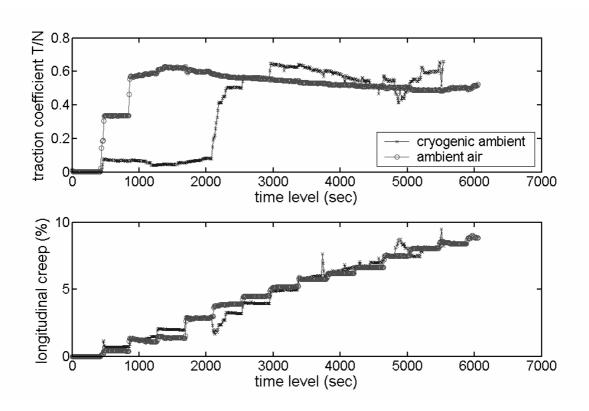
Figure 2: Longitudinal creep (slip rate) and traction coefficient T/N versus time respectively imposed and measured during the twin disc experimentation in ambient air and in cryogenic ambient. Ambient air test is marked by (o) and cryogenic ambient test is marked by (x).
