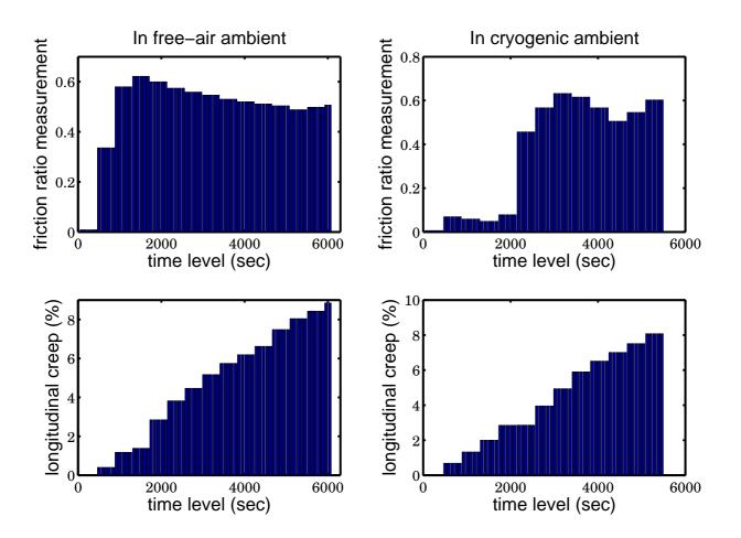
Figure 8: Modelling of the creepage history during the wear experiment and corresponding modelled coefficient of friction used for the numerical simulation of the wear evolution during the test. In Ambient air case and in liquid Nitrogen case. The second experiment duration is a little shorter.
