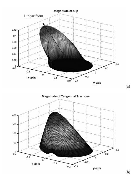
Figure 5: Steady state rolling contact twin disc problem solved using Fastsim approximation. One can observe a large adhesive zone (larger than the reference solution of Fig. 4). The relative speed  $w_x$  is linear in the slipping zone (a). The tangential traction  $\tau_x$  is linear in the adhesive zone (b). Both distributions are very similar to the reference solution and give less than 1% difference on the dissipated power  $P_d$  during rolling.
