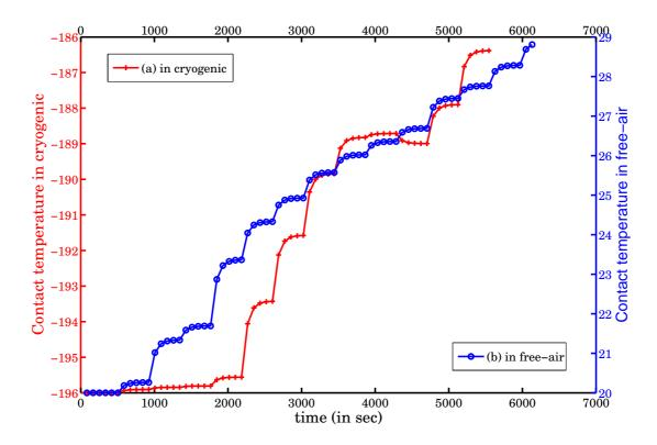
Figure 13: Temperature evolution during twin-disc experiment (numerical simulation). Case (a) ambient air condition,  $T_{\infty} = 20^{\circ}$ C. Case (b) cryogenic condition,  $T_{\infty} = -196^{\circ}$ C. In both cases increase of temperature does not exceed 10°C. This small increase is not sufficient to explain coefficient of friction instability during the cryogenic test.
