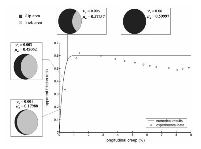
Figure 6: Apparent coefficient of friction  $\mu_a$  versus longitudinal creep for  $\mu = 0.6$ . Experimental values of ambient air test are superposed (diamonds) and follow approximately the same evolution. The partition between slipping zone and adhesive zone is illustrated for several longitudinal creepage values. When slip occurs on the complete contact area the apparent coefficient of friction  $\mu_a$  is equal to the real coefficient of friction  $\mu$ .
