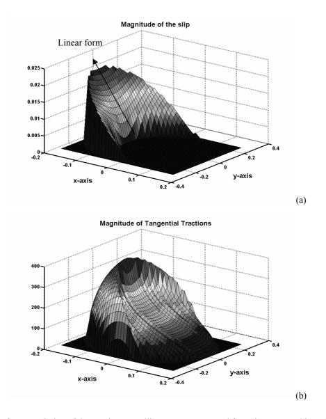
Figure 4: Reference solution of the steady state rolling contact computed from the exact problem. One can observe the linearity of the relative speed  $w_x$  in the slipping zone (a). In the adhesive zone, one can observe the non linear evolution of tangential traction  $\tau_x$  (b).
