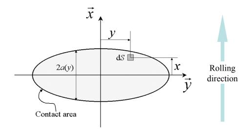
Figure 10: Description of the contact area in Hertzian problem. The rolling direction is x-direction
