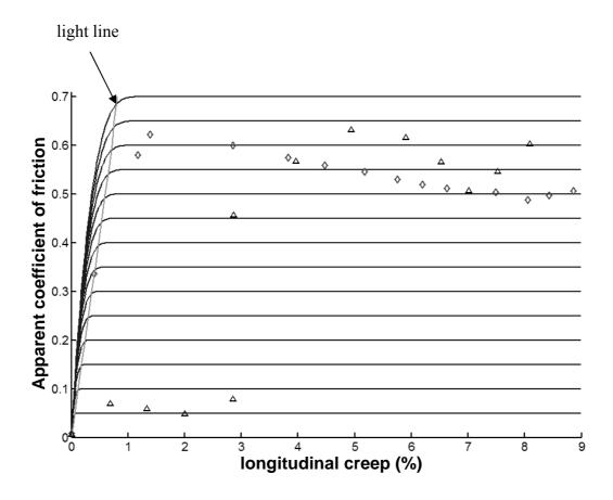
Figure 7: Friction coefficient versus longitudinal creep identification chart. Guide lines are plotted for  $\mu$  values varying from 0.05 to 0.7 step of 0.05, measured coefficient of friction are given by diamonds for air conditions and triangles for cryogenic conditions. One can observe that the coefficient of friction is very small in cryogenic conditions until longitudinal creepage remains less than 3%.
