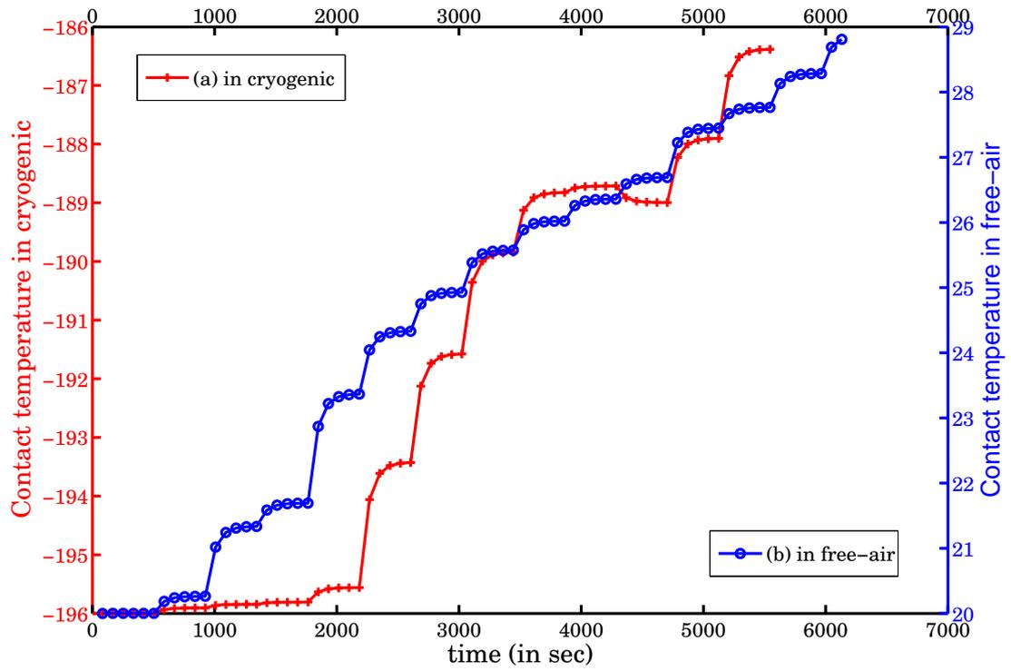
Figure 13: Temperature evolution during twin-disc experiment (numerical simulation). Case (a) ambient air condition,  $T_{\infty} = 20^{\circ}\text{C}$ . Case (b) cryogenic condition,  $T_{\infty} = -196^{\circ}\text{C}$ . In both cases increase of temperature does not exceed  $10^{\circ}\text{C}$ . This small increase is not sufficient to explain coefficient of friction instability during the cryogenic test.
