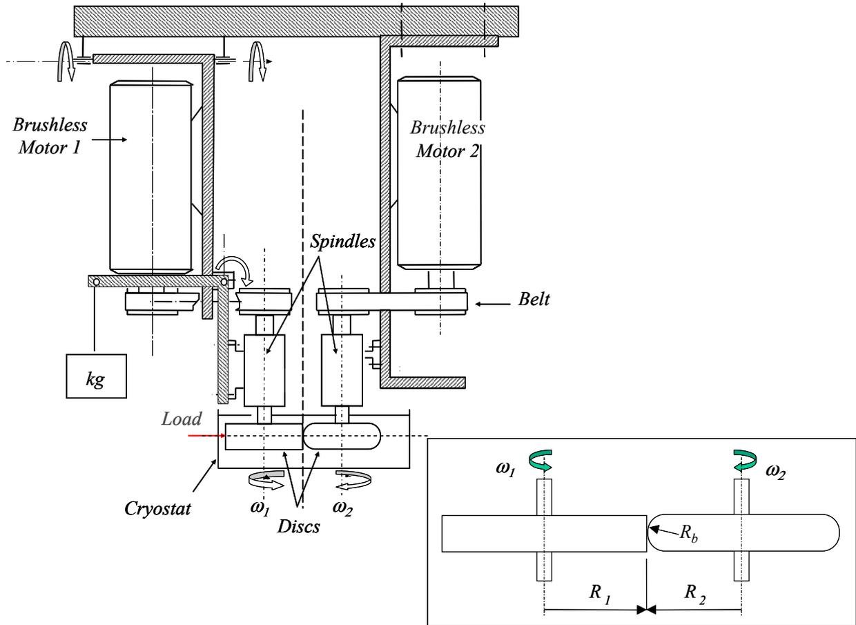
Figure 1: Twin-disc apparatus. Rotation rates are imposed to both discs and slip can be controlled. Normal load  $N$  between the two discs is constant during the test and tangential load  $T$  is measured continuously. Rotation rate is about 3000 rpm. The rolling velocity of the contact point is about 9.5 m/s.
