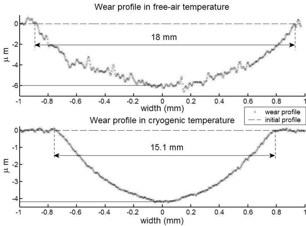
Figure 9: Rolling zone profile for disc 1 after the experiment for  $N = 72\text{N}$  in ambient air (top) and in Liquid nitrogen condition (bottom). One can see that wear depth is lower for cryogenic condition than for ambient air condition, which is easily justified by the lower value of the mean coefficient of friction during that test and the smaller duration.
