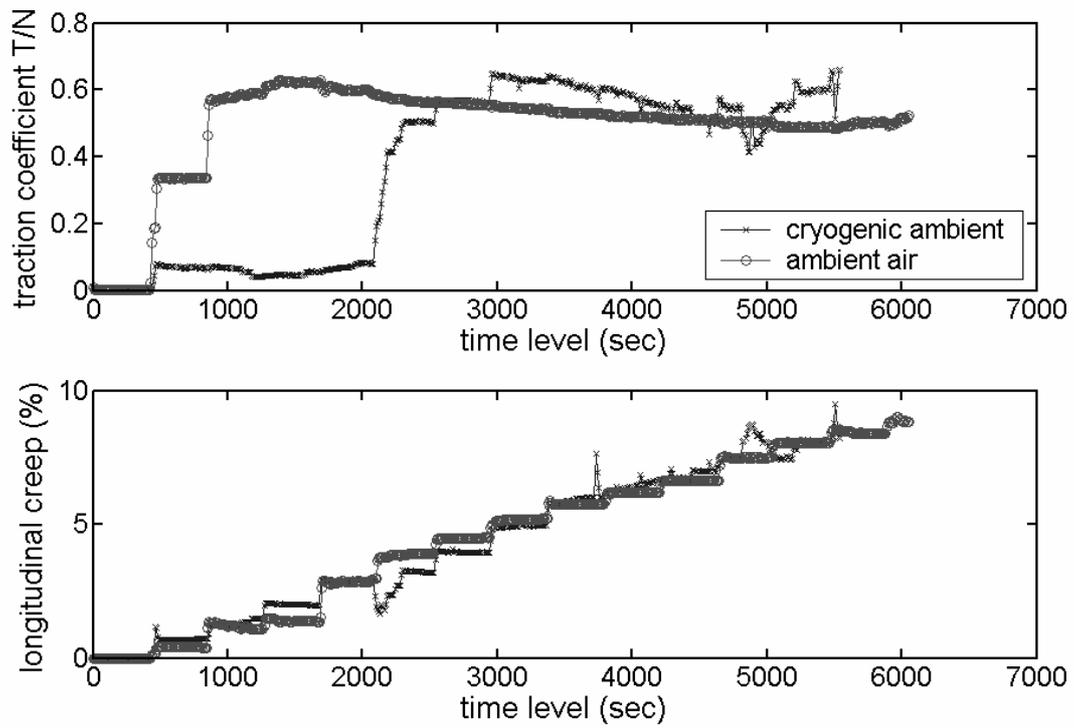
Figure 2: Longitudinal creep (slip rate) and traction coefficient  $T/N$  versus time respectively imposed and measured during the twin disc experimentation in ambient air and in cryogenic ambient. Ambient air test is marked by (o) and cryogenic ambient test is marked by (x).
