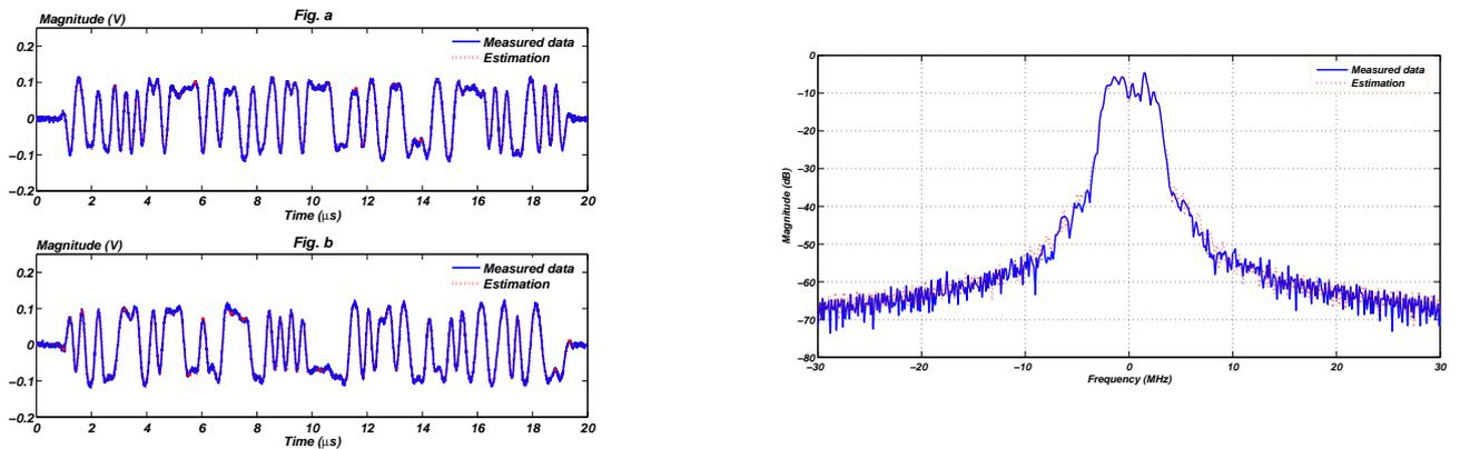
Fig. 7. (a) Time-domain measurement and estimation for QPSK modulation (b) Measured and estimated output spectrum
