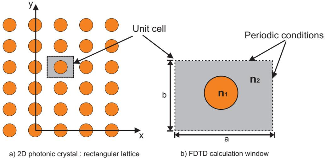
Figure 9.6: Rectangular structure and FDTD window calculation
