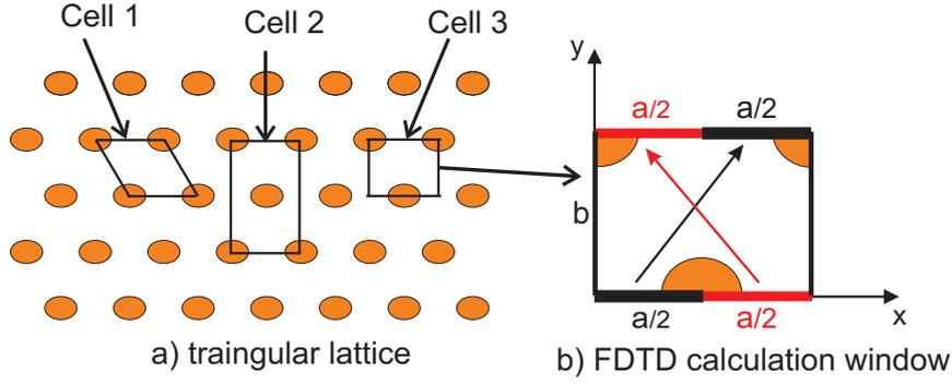
Figure 9.7: Triangular structure and FDTD calculation window
