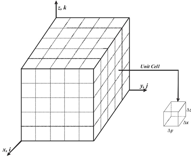
Figure 9.1: An exemple of the FDTD calculation volume.
