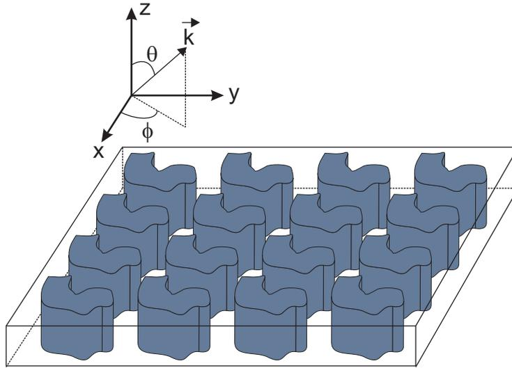
Figure 9.15: Sketch of the biperiodic structure illuminated by plane wave propagating along the  $\vec{k}$  vector defined by its Euler angles  $\theta$  and  $\phi$ .
