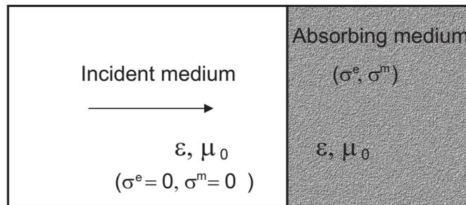
Figure 9.4: Impedance matching principle.
