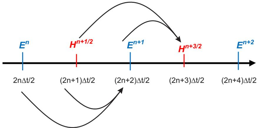
Figure 9.3: Temporal discretization into the Yee's scheme.
