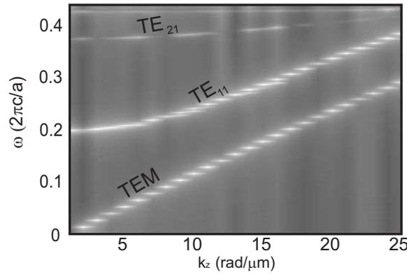
Figure 9.13: Dispersion curves at  $\Gamma$  point for the coaxial structure made in silver (lattice constant  $a = 160$  nm, inner radius  $r_i = 50$  nm and outer radius  $r_e = 75$  nm; silver dispersion is modeled by a Drude model).
