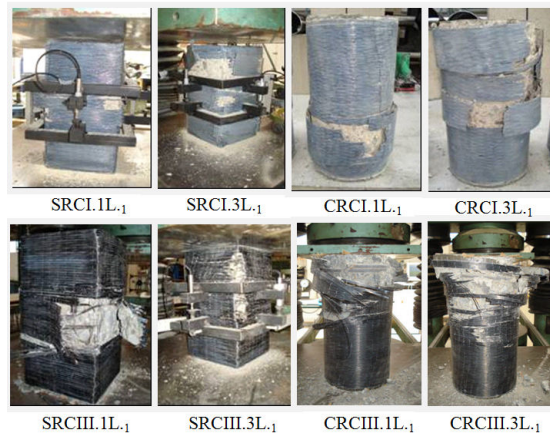
Figure 11. Typical failure modes for the tested specimens
