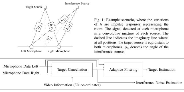
Fig. 2: System overview that shows the two main stages to the algorithm; target cancellation that produces a noise reference, and the adaptive filtering stage which recovers the target source. The work in this paper assumes that the location and the 3D co-ordinates of the speaker are known.
