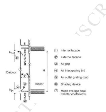
Figure 1: Schematic diagram of a double skin façade according to Faist [22].
