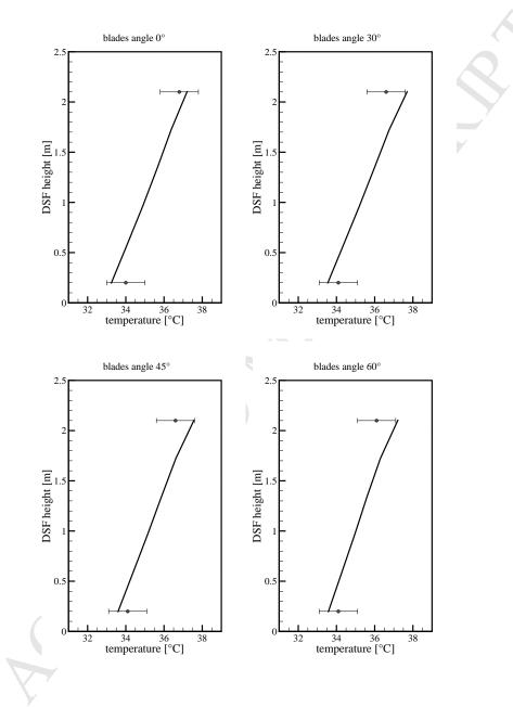
Figure 11: Air temperature profile in the right channel of the DSF for an airflow equal to  $400m^3h^{-1}$  - circle: experimental data and line: numerical modelling.
