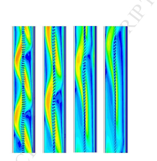
Figure 2: Isotherm zone in a DSF predicted by CFD - Extracted from [20].
