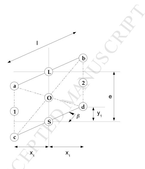
Figure 4: Hottel method applied to the double skin façade: e = 0.025m spacing between the blinds, l = 0.025m blind's width and  $\beta$  blind's angle.
