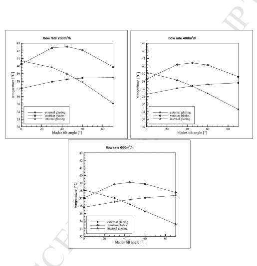
Figure 13: Temperature variation in the DSF for different air flows and blades tilt angles - Numerical modelling.
