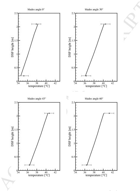
Figure 12: Venetian blades temperature for an airflow equal to  $400m^3h^{-1}$  - circle: experimental data and line: numerical modelling.
