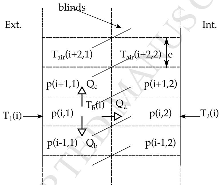
Figure 3: Double skin façade layers discretization and variables.
