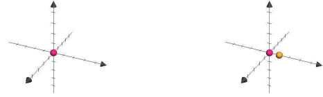
Figure 3. U(1, x) = U(1) = [1, -1, 2, -2, 3, -3, 0] means that the first axis of segmentation is x -axis and the direction is +1
