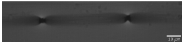
Fig.9. Effective repulsion between two nickel microspheres subjected to an external magnetic field of an intensity H_0=16\text{ kA/m} and parallel to the line connecting the centers of both microspheres. The volume fraction of the (S)-nanoclusters is 0.16%
