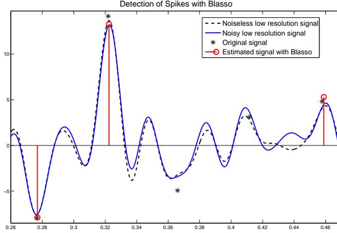
FIGURE 1. The problem is the following: we aim at recovering some spikes of the original signal (stars  $*$ ) from the observation of a corrupted optical device (blue line) which can differ heavily from the true noiseless observation (black dotted line). Our procedure (red circles) provides a close estimate of the location of some spikes.
