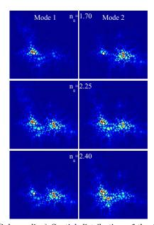
Fig. 2. (Color online) Spatial distribution of the field amplitude for  $\text{Mode}_1$  and  $\text{Mode}_2$  of Fig. <u>1</u> for three different values of the refractive index of the scatterer located at the white spot. Media 1 displays the evolution of the mode profiles as  $n_s$  increases from 1.05 to 2.40.
