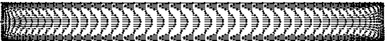
FIG. 1. Velocity vector field for the flow induced by an ultrasound source with H_b = 0.8 and A = 5200 in a two-dimensional cavity with aspect ratio A_x = 10 .
