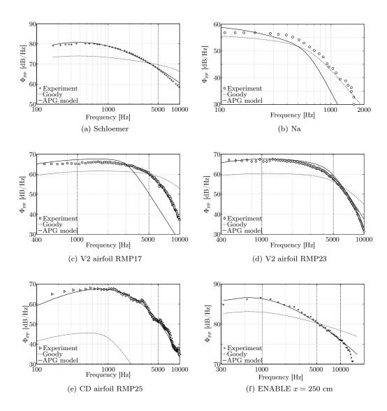
Fig. 17: Wall pressure spectra. Comparison between Goody's model and present model.
