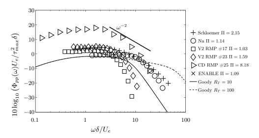
Fig. 14: Wall pressure spectra normalized by mixed variables using  $\delta$ . APG spectra compared with Goody's model.
