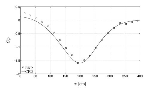
Fig. 5: Wall pressure coefficient along the streamwise direction at the bottom side of the test section.
