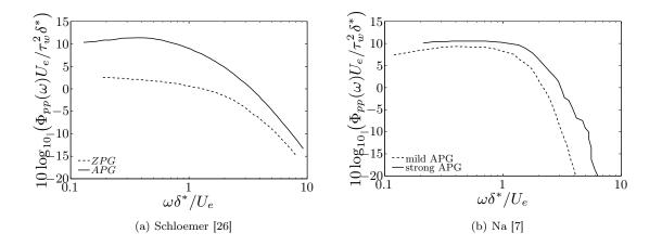
Fig. 4: Wall-pressure spectra scaled with mixed variables: adverse pressure gradient (APG) effect.
