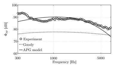
Fig. 19: Wall pressure spectrum in the aft region of a NACA5510 profile. Comparison between Goody's model and present model.
