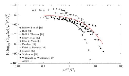
Fig. 1: Wall pressure spectra scaled by outer variables. Amiet's WPS model [1] vs data collected by Keith *et al.* [15] and corrected for spatial resolution errors.
