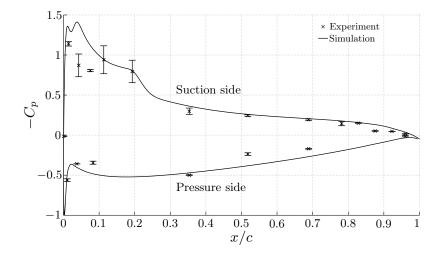
Fig. 9: Mean pressure coefficient (-Cp) on V2 airfoil.
