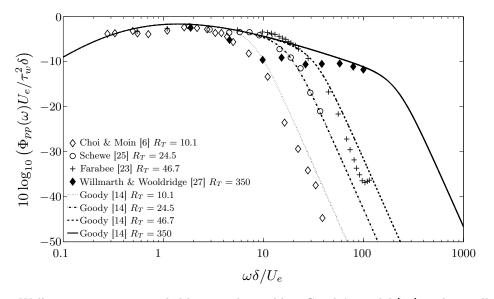
Fig. 3: Wall pressure spectra scaled by mixed variables. Goody's model [14] vs data collected by Keith *et al.* [15] and corrected for spatial resolution errors.
