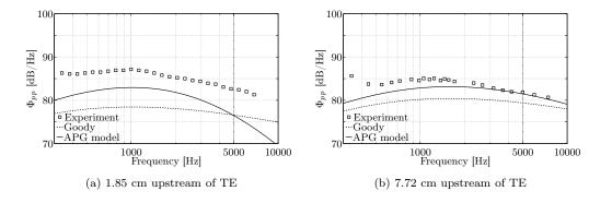
Fig. 20: NACA0012 wall pressure spectra. Goody's model, present model and experiments by Brooks & Hodgson [56].
