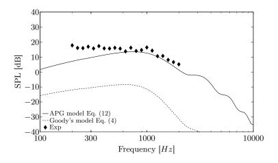
Fig. 18: Far field acoustic spectra in dB (integrated over 8 Hz bin width and reference to  $2 \times 10^{-5}$  Pa) in the midspan plane above the CD airfoil at a distance of 2 m. Experiment from Moreau & Roger[34] is compared to Amiet's model.
