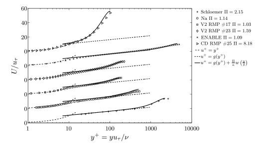
Fig. 13: Velocity profiles in wall units.
