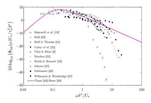
Fig. 2: Wall pressure spectra scaled by mixed variables. Chase [28]-Howe [29] model vs data collected by Keith *et al.* [15] and corrected for spatial resolution errors.
