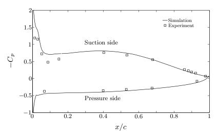
Fig. 11: Mean pressure coefficient (-Cp) on CD airfoil.
