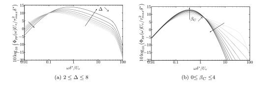
Fig. 16: Evolution of the wall-pressure spectral model with the adverse pressure gradient
