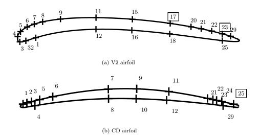
Fig. 8: Remote Microphone Probes (RMP) positions on airfoils.
