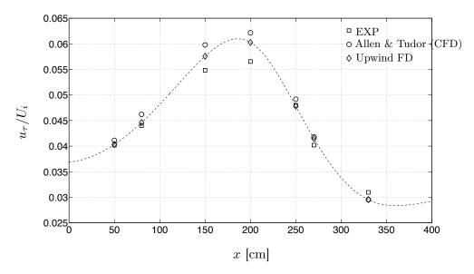
Fig. 7: Friction velocity normalized by the inlet velocity. Experimental results (Weiser probe) compared with upwind finite difference (FD) and Allen & Tudor's method.
