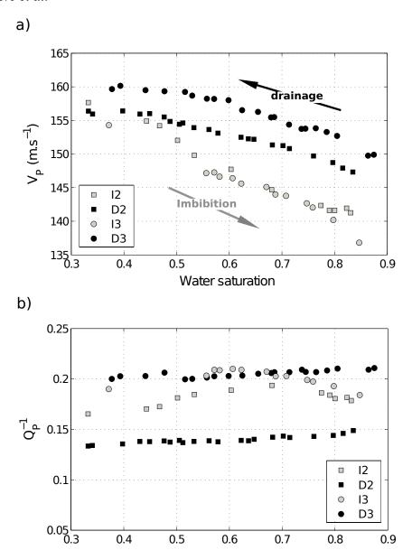
Figure 6. a) Measured P-waves phase velocity  $V_P$  and b) inverse quality factor  $Q_P^{-1}$  as a function of  $S_w$ , recorded during the second imbibition I2, the second drainage D2, the third imbibition I3 and the third drainage D3, for f = [1.6 - 1.8] kHz. The arrows in a) indicates that imbibition results in increasing  $S_w$  in time whereas drainage results in decreasing  $S_w$ . The experimental error-bars at each data point are shown in Figure 7.
