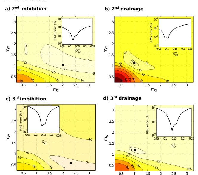
**Figure 8.** Least-square inversion residuals for  $Q_{K_D}^{-1}$ , and least-square inversion residuals maps  $(m_g, m_w)$  for the best  $Q_{K_D}^{-1}$ . The residuals are shown for the experiment I2, D2, I3, D3 in a), b), c) and d) respectively. The effective pressure is varying for I2 and I3 in a) and c), and is constant for D2 and D3 in b) and d) (see Table 3).
