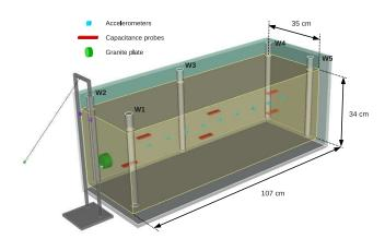
**Figure 2.** Schematic view of the experimental set-up. A steel ball mounted on a pendulum hits a circular granite plate on the left lateral side of the sand-filled tank. Wave propagation is monitored by nine aligned buried accelerometers. Water saturation level is measured by capacitance probes. Five wells W1-W5 are used to proceed to imbibition or drainage.
