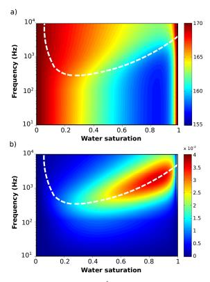
Figure 1. a) Phase velocities  $V_P$  in m/s and b) inverse quality factors  $Q_P^{-1}$  as a function of the frequency and the water saturation. The computations are performed using Biot's theory extended to an effective fluid and Walton's model to estimate  $K_D$ . The physical parameters of this calculation are given in Table 2. Biot's frequency in dashed white line in both figures varies with the water saturation since it depends strongly on the effective fluid density and viscosity.
