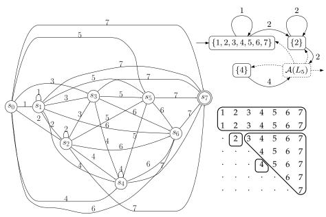
**Fig. 1.** The reduced automaton (at right) is obtained from a decomposition transition table (at right bottom) of the homogeneous automaton (at left). The automaton  $\mathcal{A}(L_5)$  is the part of the reduced automaton which represents the triangle (in the transition table decomposition).
