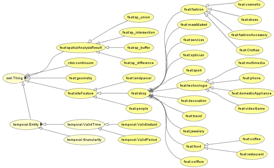
Fig. 7. Class hierarchy of the ontology (using protégé plug-in OWL viz-Tab)
