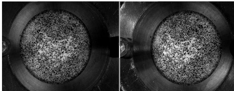
Fig. 3 View of the specimen layer during the inflation test through the left and right cameras
