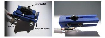
Fig. 6. Module for one finger containing the lever-switch and pressure sensors and a vibrator.
