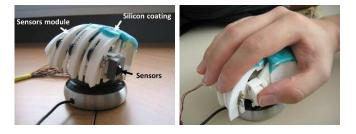
Fig. 7. Final prototype V4.
