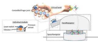
Fig. 8. Schematic design of the final prototype V4.
