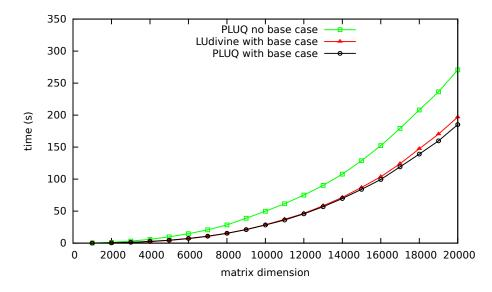
Figure 4: Computation time with dense rank deficient matrices (rank is half the dimension)
