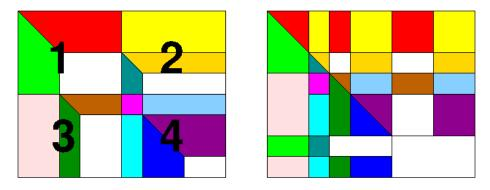
Figure 1: Block recursive Z-curve PLUQ decomposition and final block permutation.
