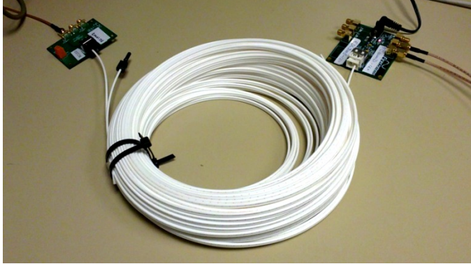
Figure 2. Commercially available electro-optical components and 50-m SI-POF
