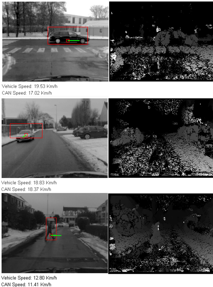
Fig. 25 Confirmed objects. The top figure illustrates the visual confirmation of a highly dynamic object (Scenario B in Fig. 23). The middle figure shows a vehicle having just turned. Here the ROI is delocalized because of pitch changes, given that the ego-vehicle is accelerating (Scenario C in Fig. 23). The bottom figure shows the confirmed pedestrian when crossing the road in Scenario E (Fig. 23)
