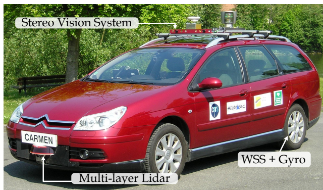
Fig. 3 The experimental vehicle with the stereo vision system and the IBEO Alasca XT. (Velodyne is not used in this study)
