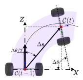
Fig. 8 Yaw rate-WSS dead-reckoning for planar odometry estimation
