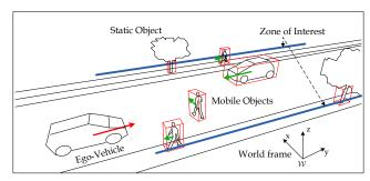
Fig. 1 A Dynamic Map is composed of a list of the states of tracked objects located within a zone of interest together with the changing vehicle dynamics in the 3D scene.
