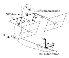
Fig. 5 The multi-sensor frames are located at the optical center of the left camera,  $\mathcal{G}$ , the midpoint of the SVS,  $\mathcal{S}$ , and the ML-lidar sensor,  $\mathcal{L}$ .
