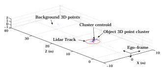
Fig. 20  $\,$  3D visualization of a confirmed track using 3D point clusters
