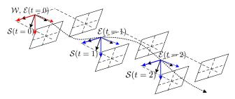
**Fig. 9** World (W) and Ego ( $\mathcal{E}(t)$ ) and SVS ( $\mathcal{S}(t)$ ) frames at 3 sampling times
