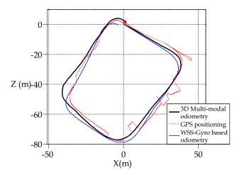
Fig. 10 Bird's eye view of the 3D Reconstructed Trajectory compared to WSS-Gyro odometry and GPS positioning
