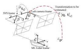
Fig. 11 Extrinsic Camera- Multi-layer Lidar Calibration
