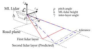
Fig. 13 Road lidar data filtering
