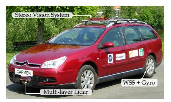
Fig. 3 The experimental vehicle with the stereo vision system and the IBEO Alasca XT. (Velodyne is not used in this study)
