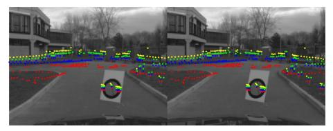
Fig. 12 ML Lidar data re-projection on stereo images
